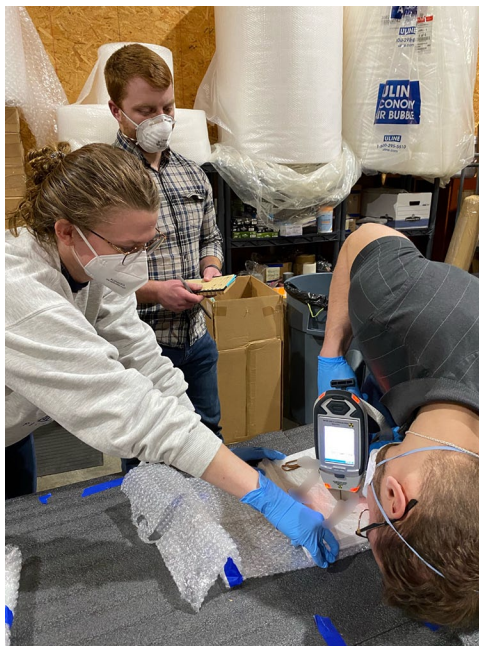
Figure 4. With permission from tribal authorities, the student team uses XRF technology to test collections for heavy metal contaminants before the items are repatriated to tribal communities.
